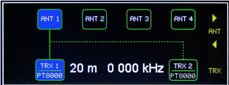
Fig. 8-3: Antenna Allocation – Factory Setting
