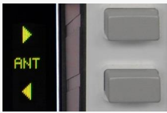
Fig. 8-2: Antenna Allocation – Change of Antenna Connector
