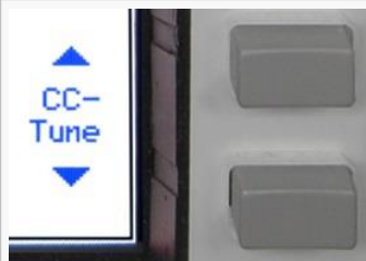
Fig. 8-19: Manual Tuning – Center Capacitance CC
